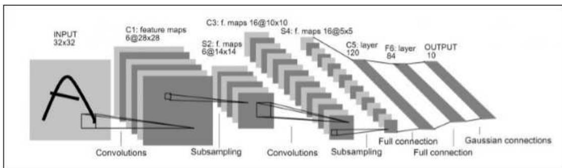
**Figure 4: The Structure of the LeNet Neural Network.**
